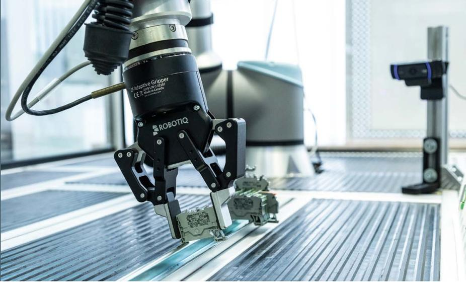
implemented in the framework control the robot so that it learns the underlying assembly process in the simulation through trial and error – without using or possibly damaging a single, real component. Artificial intelligence takes over the programming of the robot, even enabling the above-mentioned control cabinets to be assembled.
